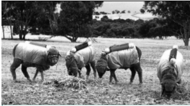
Australian sheep have been fitted with methane-catching "backpacks" to measure the efficacy of vaccinations. The vaccinations are intended to reduce populations of methane-producing micro-organisms in sheep.
